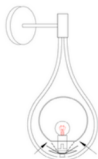
7. Clamp the triangle fork, clip the triangle fork into the glass lampshade, and loosen it gently
