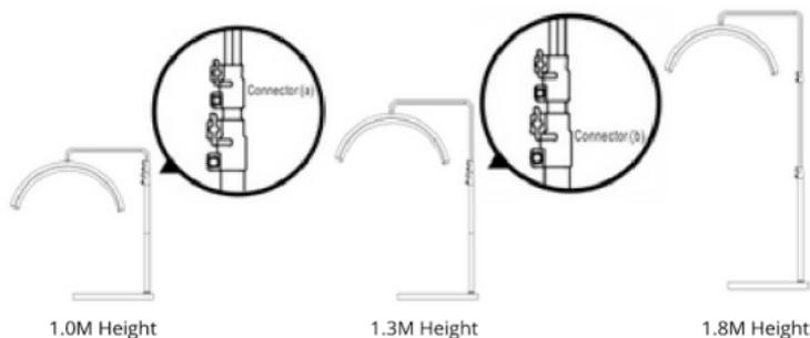
2. Set up position should have Moon Light (BASE) and Base (Part C) in the same direction for stability and safe use.
